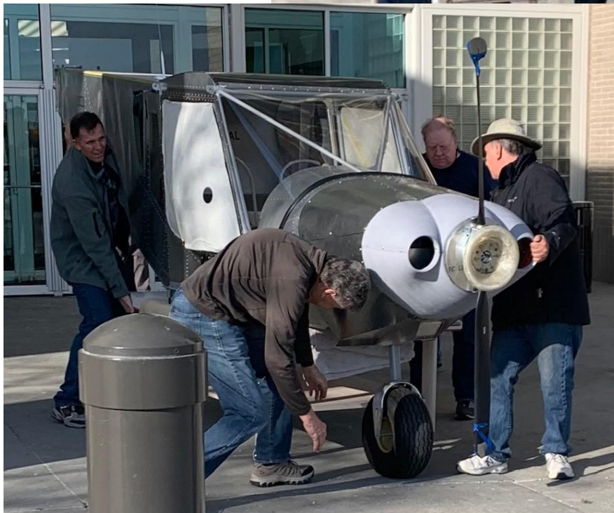
Getting the Zenith's landing gear attached.
