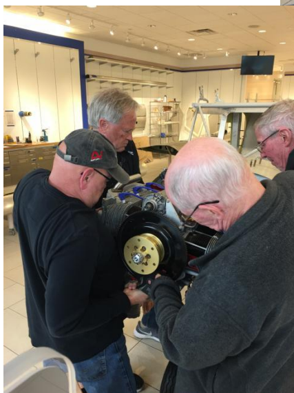
Above, left, right: Getting the Corvair engine hung on the Chapter Zenith.
