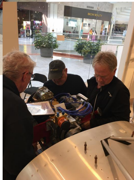
Above, left, right: Getting the Corvair engine hung on the Chapter Zenith.
