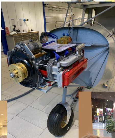
Above, left, right: Getting the Corvair engine hung on the Chapter Zenith.
