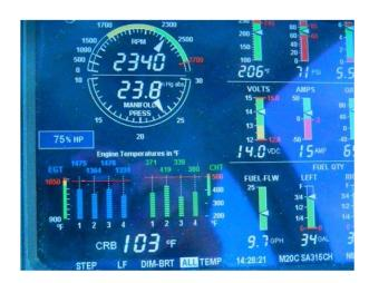
Now note that cylinders 1 and 3 have higher EGTs than cylinders 2 and 4. However the reverse is true for the CHTs, with 1 and 3 being significantly lower than 2 and 4. Note also that the Carburetor Air Temperature
