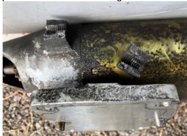
The bolt is a 5/16-18 drilled-head Lycoming
