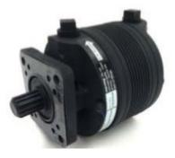
To remove the old vacuum pump, you will need a standard 7/16" combination wrench for the upper and right hand nuts, and the special Rapco Vacuum Pump Wrench, Spruce p/n 10-13911 for \$23.50 for the lower inside nut. Without this tool, your only option is to remove the entire oil filter assembly from the back of the engine, a minimum 2-hour job that will require new gaskets for reinstallation.
