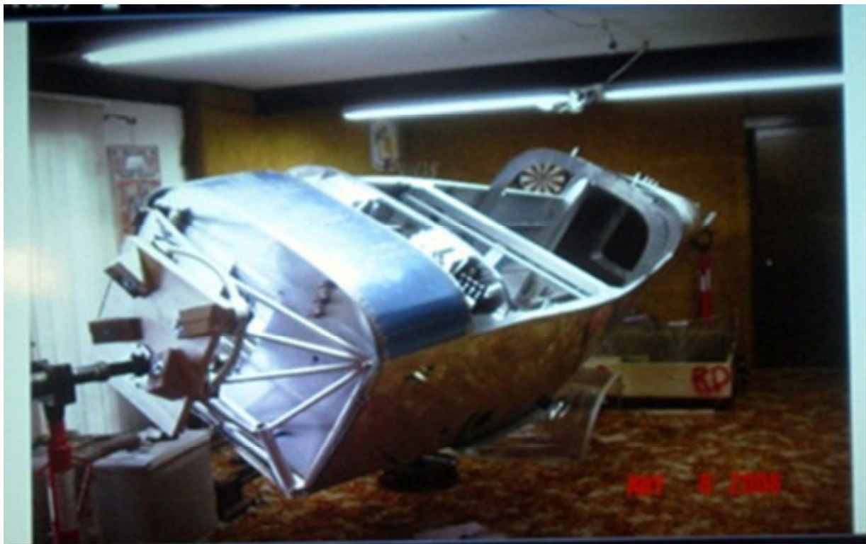
This is what Bob Cartwright's plane looked like at the last "Tour of Member Projects". Notice that the plane is on a rotisserie so Bob could rotate it to work on different sections. Photo from Dick Austin.
