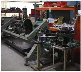
This is what a Merlin engine out of a Mustang looks like when it is all taken apart. The thing on the right is the 300hp supercharger. Maybe I could put that in my Cherokee 180!
