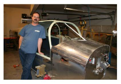
Just finished final install of the cabin top which finishes out the RV-10 fuselage kit.
